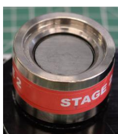
Two photographs showing how to place the backing in stage 2, zigzag side facing up for pinback buttons, and open side facing down for magnets.
