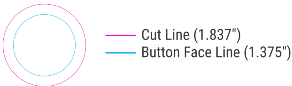
A diagram showing the Cut Line in pink and the Button Face Line in blue.
