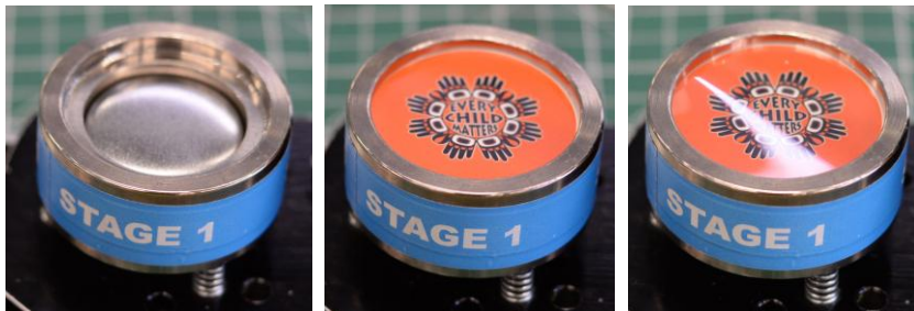
A series of photographs showing how to (1) place the convex metal shell, (2) place your cut design, and (3) place a Mylar circle.
